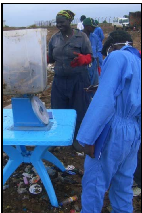
Picture 2 – weighing of waste and bulk density calculations on-going during the sampling exercise.
