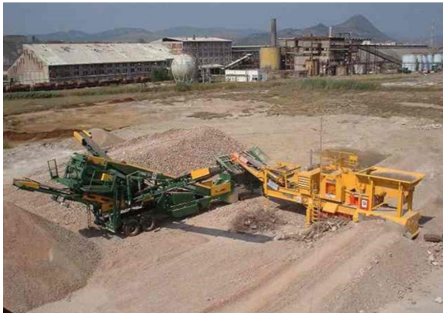
Figure 2: Typical debris recycling operation with a debris crusher (yellow) and a screening unit (green)
