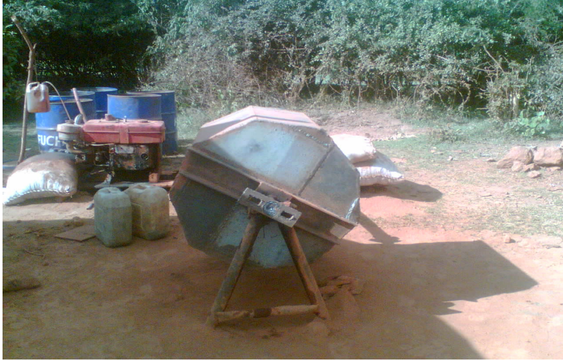
Figure 2: Local ball mill for grinding the mined ore
