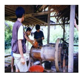
Adding mercury to the mixture of ores and water.
