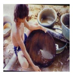
Residue after panning operation where most of the water are removed.
