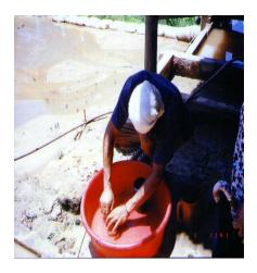
Placing of residue in filter cloth to remove the mercury from the residue.
