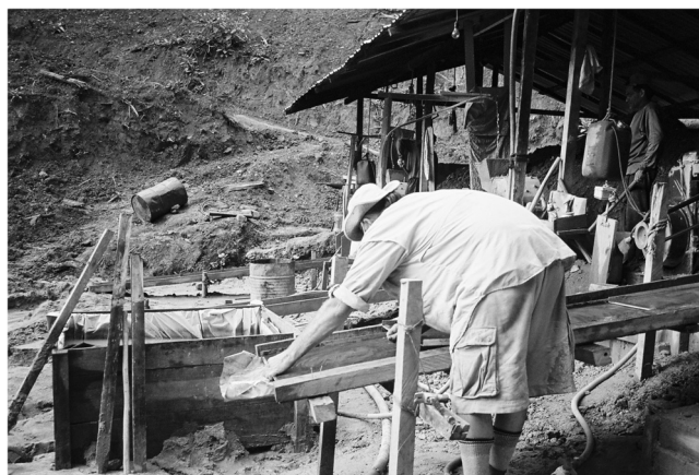
Figure 11. Example of Cleangold® test system (front) replacing copper amalgamation plates seen in the background at a hard-rock ore operation in Suriname, where the ore is prepared with a hammer mill. Assaying of a sample of the concentrates from the first of the four sluice inserts used showed almost 14 000 g gold/ton after a 24 h period of use. Photo: Kristina Shafer, www.artminers.org .
