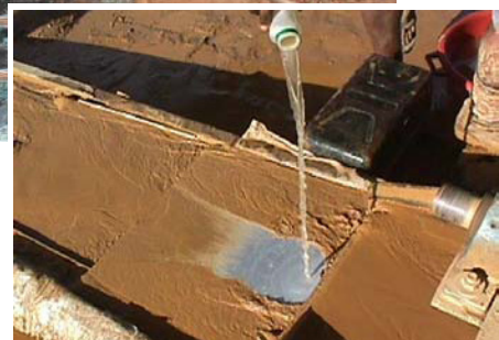
The use of copper plates for whole ore amalgamation in the Tapajós River Basin. Photo: Global Mercury Project
