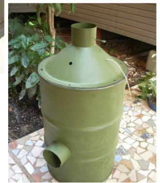
Above: The Mercury Capture System, shown being installed in a gold shop in Peru, can reduce mercury emissions by as much as 80%. Right: A prototype of the MCS before being field tested by the U.S. EPA and National Argonne Laboratory. Photos courtesy of the U.S. EPA.
