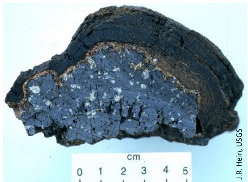
Ferromanganese crust on basalt (photo by J.R. Hein, USGS, cruise L5-85-NC, D33-1, Gorda Ridge, NE Pacific).
