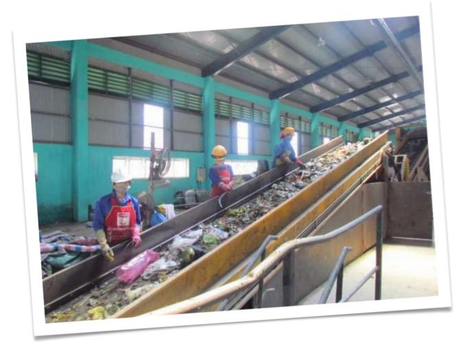
• This is modern line, linked with input which is domestic waste separated at source in developed countries like Belgian, EU. With feature of domestic waste which is not separated at source, all of waste mixed and covered by nylon and tropical climate, so the line is not exploited effectively waste treatment as desired. At those factories, performance is only from 20% to 30%.
