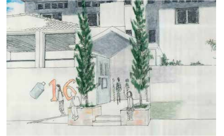
Figure 4: Example of an entry that combines steps, ramps and an informal waiting area to make sure no one is excluded from this school because of their mobility requirements
