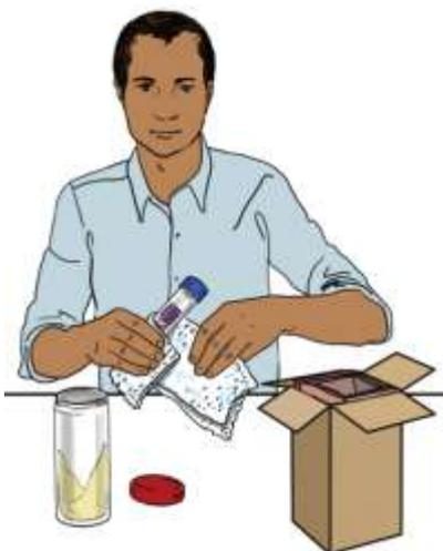
**Step 3e: Place the primary container(s) into the secondary container**
